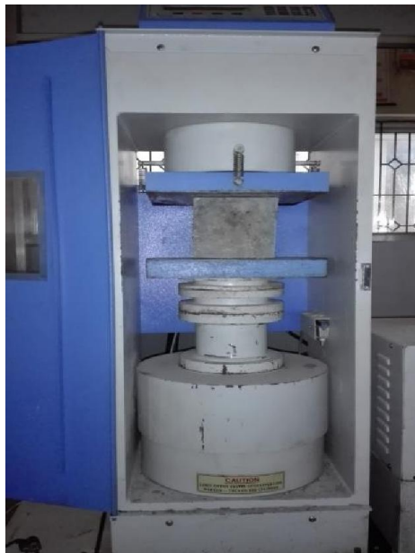
Fig 7.1 Compressive strength testing of cube Specimen
