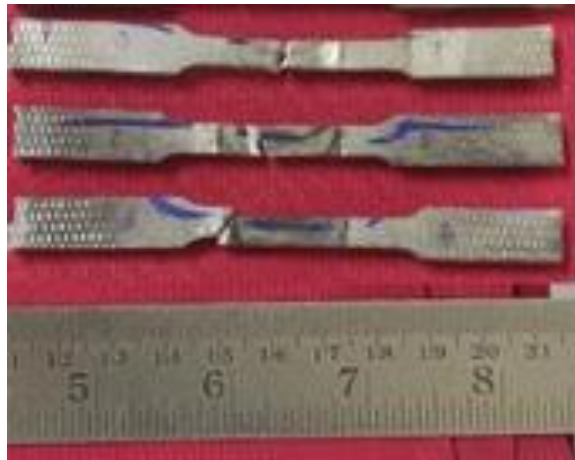
Figure 1: Tensile samples of the FSP (Mg AZ31B/Al 2 O 3 /Cu)
