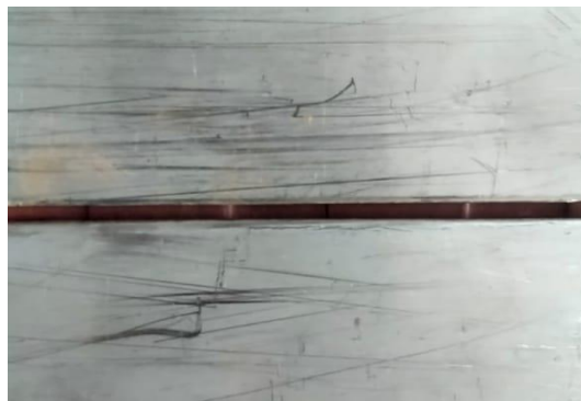
Figure 2: AISI304 SS plates (100mmx60mmx2mm)
