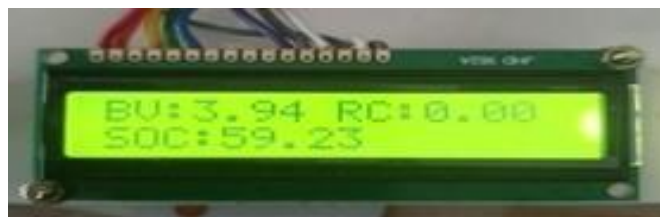
Fig 17: 60% battery in approximately 60 Min
