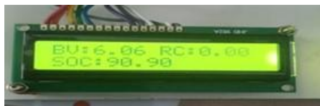
Fig 18: 90% battery in approximately 130 Min
