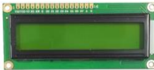
Fig 5: LCD display operating voltage 5V and 16*2=32characters.
