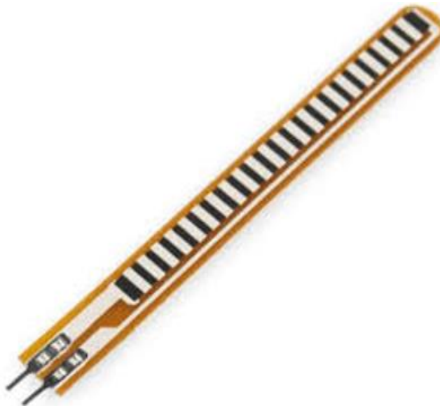
Fig 2: Flex sensor- voltage range (0-5)V dc, Power rating 0.5Watts
